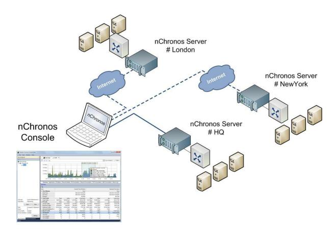
nChronos support varies network topologies to visualize all network segments from core to edge areas. nChronos can be installed at gateways, core switches, DMZ zone, critical application interfaces or critical links.
